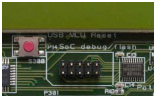
Figure 17: SmartRF04EB debug connector for debugging of external target systems
