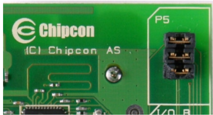
Figure 11: P5 default jumper settings
