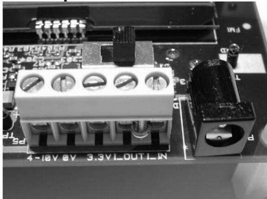
The second method applies DC power using the DC input jack (right in picture, centre is +, sleeve is ground), or by connecting a 4-10V voltage source between the 4-10V and 0V terminals of the power connector (left in picture). It is also possible to connect a 3.3V voltage source between the 3.3V and 0V terminals. The on-board voltage regulators will be bypassed in this case.
