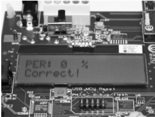
Once the PER test is ready the result will be displayed on the Sender. In this case no packets were lost.
