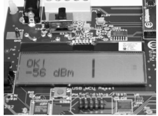
If the Sender gets the acknowledgment from the second board "OK!" and the received signal strength will be displayed.
