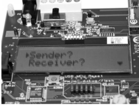
Select Sender on one EB and Receiver on the other by moving the joystick. Confirm by moving the joystick to the right. The Receiving node will display "Waiting".
