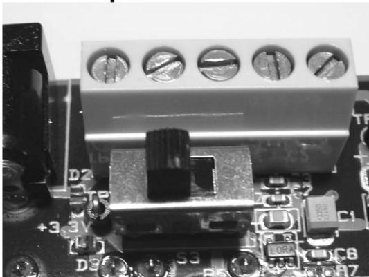
If a 3.3V source is used as described in 3b above, the switch should be set to the leftmost position. For all other cases, the switch should be set to the rightmost position. This switch can be used to turn off the EB by switching it to the opposite position of that used to turn it on.
