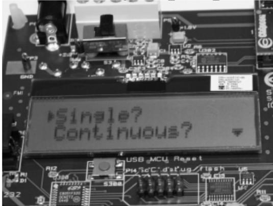
To stop the PingPong application on the Sender move and hold the joystick to the left. This will take you back to the previous menu. This time select "PER Test".
