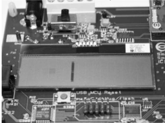
The 2<sup>nd</sup> board (Set up as "Receiver") will show a graphical presentation of the packets sent.
