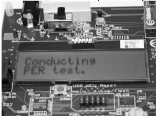
The Receiver will display "Conducting PER test" while it is sending the requested 1000 packets.
