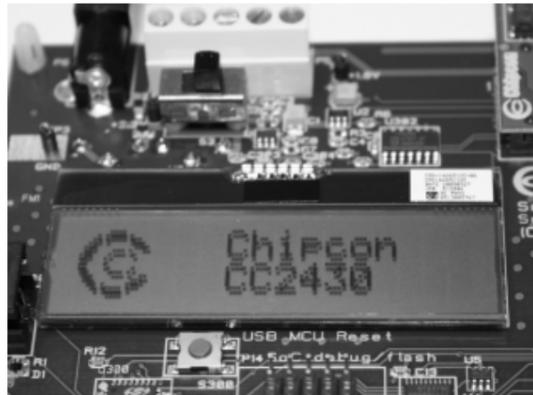
When power is applied to the board, the test program will start. You should see the Chipcon logo shown above on the LCD display on both EBs. Moving the joystick down will show the first menu item.
