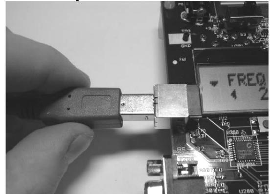
The EB can also be powered from the USB bus. Make sure that the SmartRF® Studio software is installed before connecting the EB to the PC, otherwise you may experience problems in installing it later due to driver issues.
