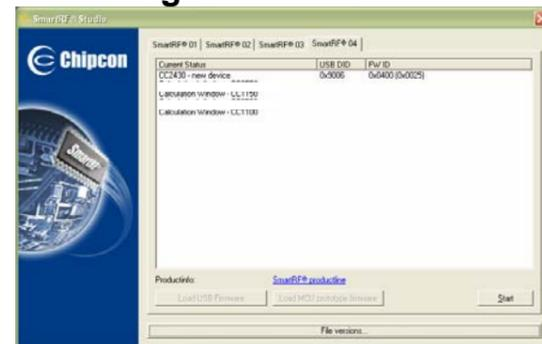
After the install program finishes, connect the EB to the PC using the USB cable. Run SmartRF® Studio. Select the SmartRF®04 tab. Select the CC2430 board, and click the Run button.
