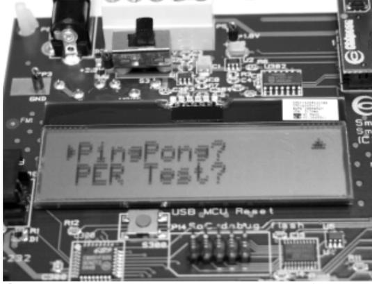
On the sender select PingPong and confirm by moving joystick to the right. The board set up to be the sender will start to send packets and the Receiver board will send back a response.
