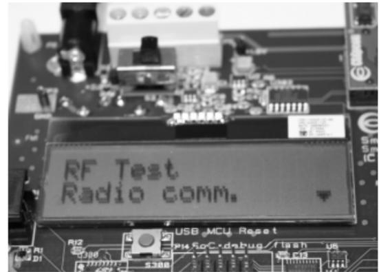
The first menu item is RF Test. Select this test by moving the joystick to the right.
