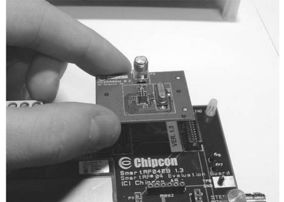
Insert a CC2430EM into both SmartRF04EBs. The connectors will only fit in one position, so that the EM cannot be inserted the wrong way. Do not force the EM.
