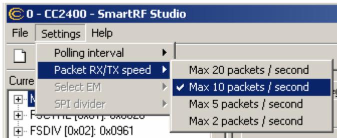
*Packet RX/TX speed* - Defines the minimum transmission interval for packet transfer in Normal View. Reduce this value in RX and TX (both!) if the number of lost packets seems unreasonably high.
