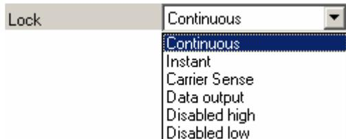
Note that the Lock indicator pin on CC102X is active low.
