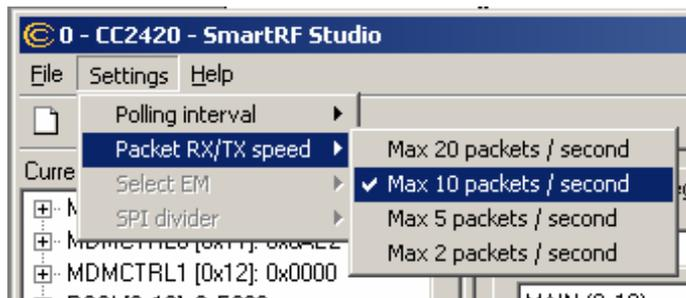
*Packet RX/TX speed* - Defines the minimum transmission interval for packet transfer in Normal View. Reduce this value in RX and TX (both!) if the number of lost packets seems unreasonably high.
