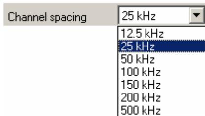
Note that CC1021 cannot be configured to 12.5 and 25 kHz narrow band operations.
