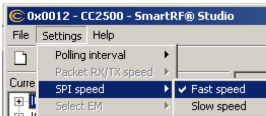
*SPI speed* - Defines the SPI communication speed between the SmartRF® 04 evaluation board and CC11xx/25xx.
