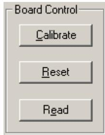
**Calibrate** activates the on-chip calibration feature of the VCO and PLL on the CC1000.
