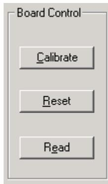
**Calibrate** activates the on-chip calibration feature of the VCO and PLL on the CC1050.
