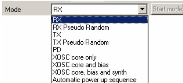
When Automatic power up sequence is selected, the CC102X wakes up in RX mode and check the carrier sense signal. The power up sequencing is initiated by a negative transition on PSEL. Pushing the 'wake up' button does this. Please refer to the data sheet for further information on power-on sequencing.
