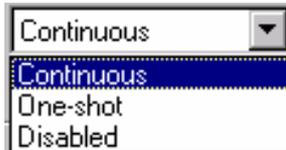
Important: The 'One-shot' lock signal is used internally in the CC900 to enable the transmitter. If the lock signal is not active (high) the transmitter will not be enabled. This is done in order to avoid the transmitter to emit out-of-band signals. If 'Disabled' is chosen this function is overridden and care should be taken, as the transmitter will transmit even when the PLL is not in lock.
