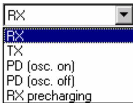
Leaving the crystal oscillator running gives a shorter turn-on time at the expense of higher current consumption in the power down mode. RX precharging can be used to reduce the demodulator turn-on time. Please refer to the data sheet for further information on demodulator precharging. The default value is RX.
