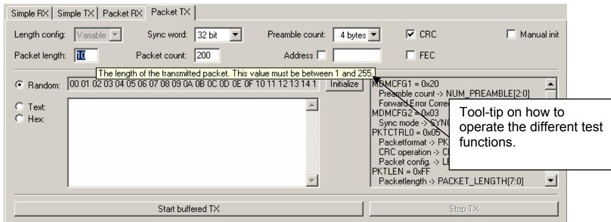
Warnings are indicated by turning the relevant control(s) yellow. One such warning will appear when choosing a sync word smaller than 32 bits in the Packet RX/TX tests in Normal View.
