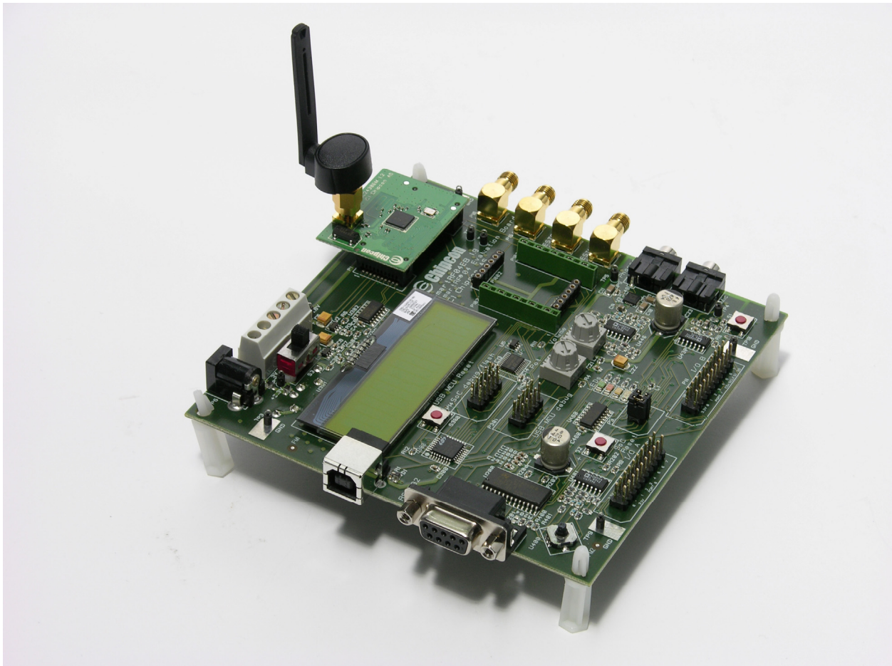
Figure 1: Chipcon SmartRF04EB Evaluation Board with CC2430EM
