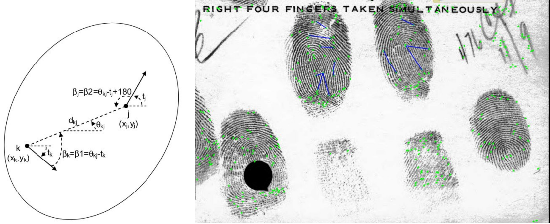
Figure 2.3: Pair-table consists of computation of relative distances and angles between minutiae points making the representation rotation and translation invariant. In the above figure shown is the concept of computation of relative distances and angles between minutiae points (figure from [3]) along with its physical interpretation on actual fingerprint (the edges are displayed in blue) This figure best if viewed in color
