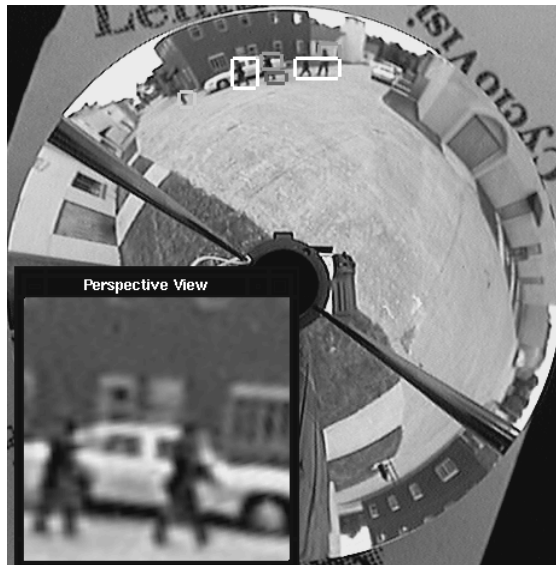
Figure 1: Tracking system with a single perspective “target” window.
