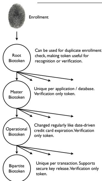
**Fig. 1.** The biotoken issue/re-issue tree. Biotokens can be re-encoded, starting from the root token generated at enrollment time, through subsequent applications of PK encryption (supporting automatic revocation and re-issue) or a hash function.
