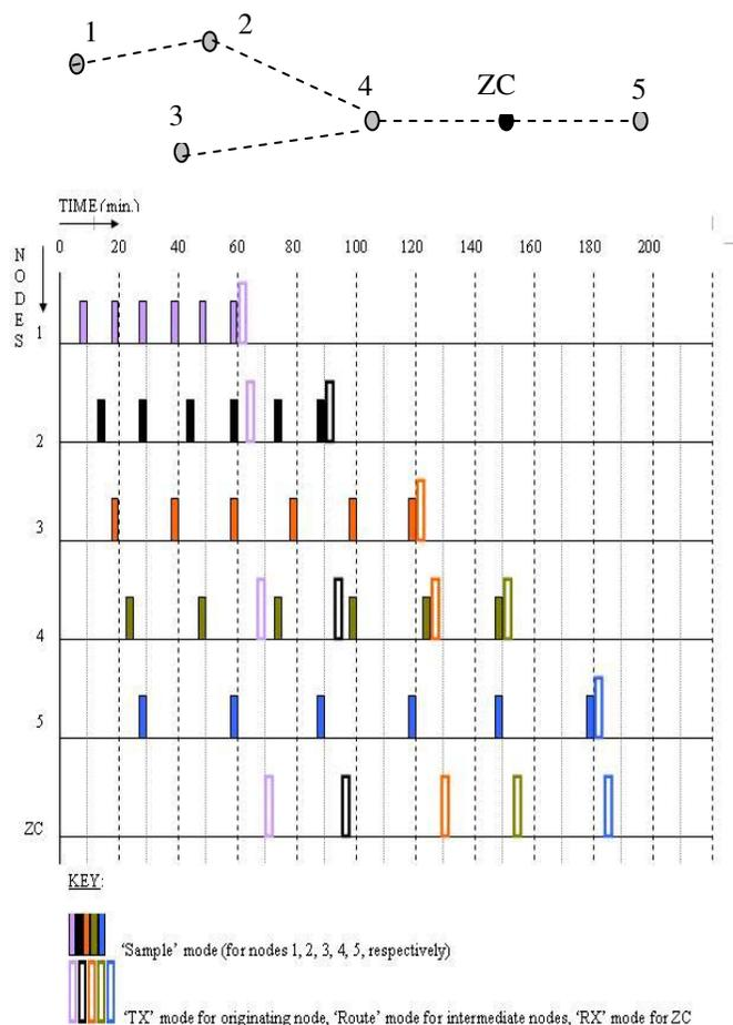
**Figure 1: A simple 6 node network, and the resulting schedule. In the example nodes 1-5 sample data every 10, 15, 20, 25 and 30 minutes respectively and must transmit their stored data every 60, 90, 120, 150 and 180 minutes respectively. The hollow bars in the schedule show when nodes wake up to support transmission of data for other nodes.**
