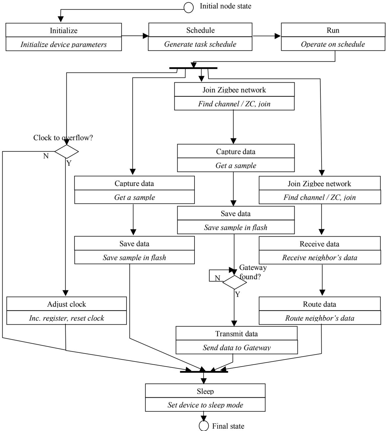
**Figure 2: Network Node State Diagram**
