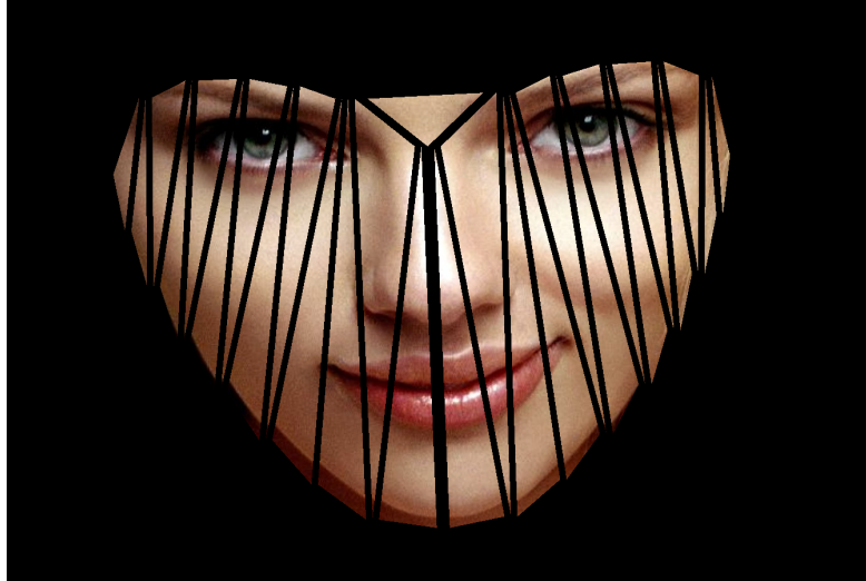
FIGURE 3.20: Via our per-pixel triangular closure in barycentric coordinates, we can efficiently manipulate triangles derived from the mesh points fit by the AAM.
