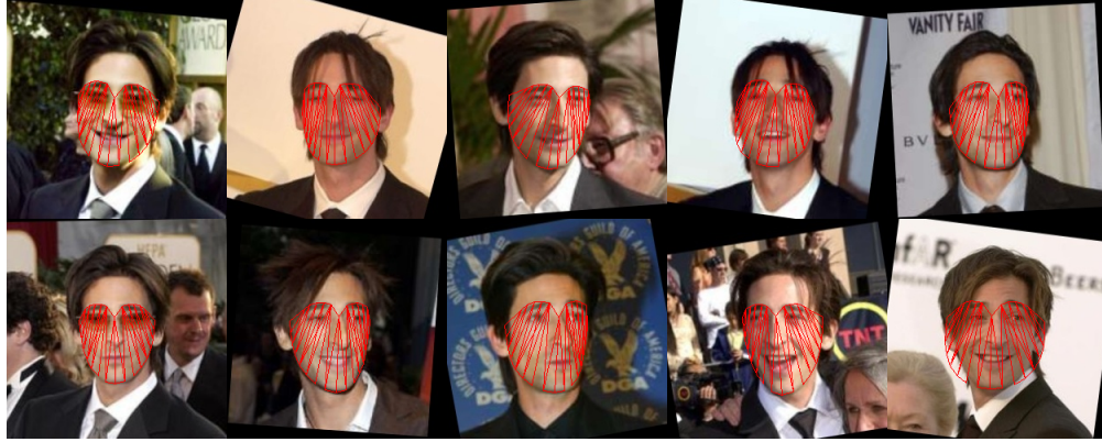
FIGURE 3.18: Note how the longitudinal triangles capture scale changes due to yaw rotations for several images of a subject from LFW. Pitch changes are also captured. However, when the AAM fit fails the associated scale information is spurious.
