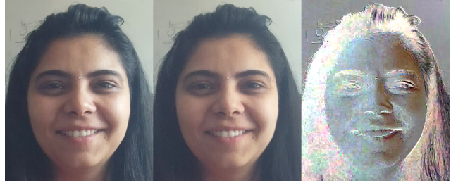
Figure 2. POLARIZATION OF A FACE. Images were obtained by manually rotating a polarizer in front of the camera of a Samsung Galaxy S6 Edge™ smartphone. Left: linear horizontal polarization. Center: linear vertical polarization. Right: PARAPH image I_P from Eq. (3). Under horizontal polarization, the intensity of specularly polarized light is noticeably greater. Note that scaling has been applied for visualization.
