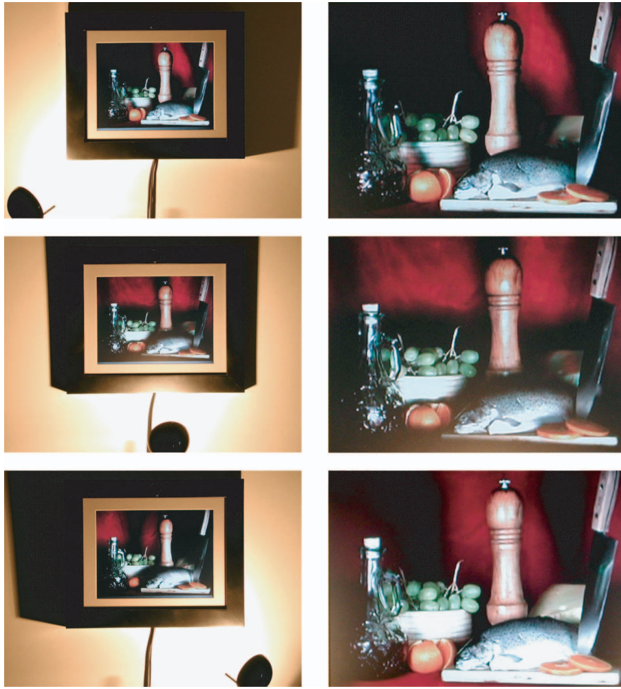
Fig. 10. LSD outputs for a still life scene with different illuminations. Note the shadows cast by the pepper dispenser, the fish and the knife; the specularities on the dispenser, knife, bottle, orange and grapes; and the textures on the fish, the grape basket and the red velvet cloth.
