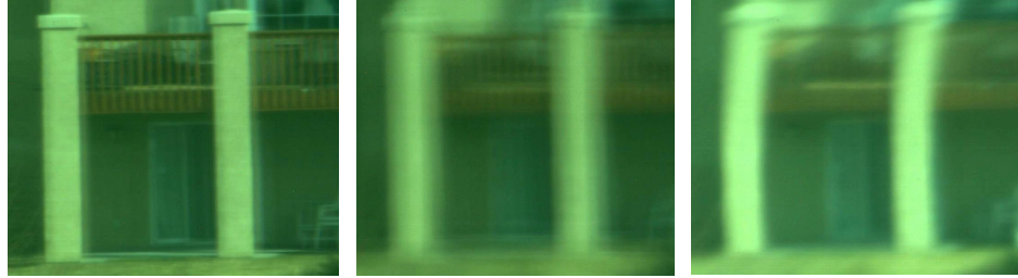
Figure 3: Imaging showing clean image, blur and distortion effects. Central 700x720 region from 2048x1520 image at 800m F8
