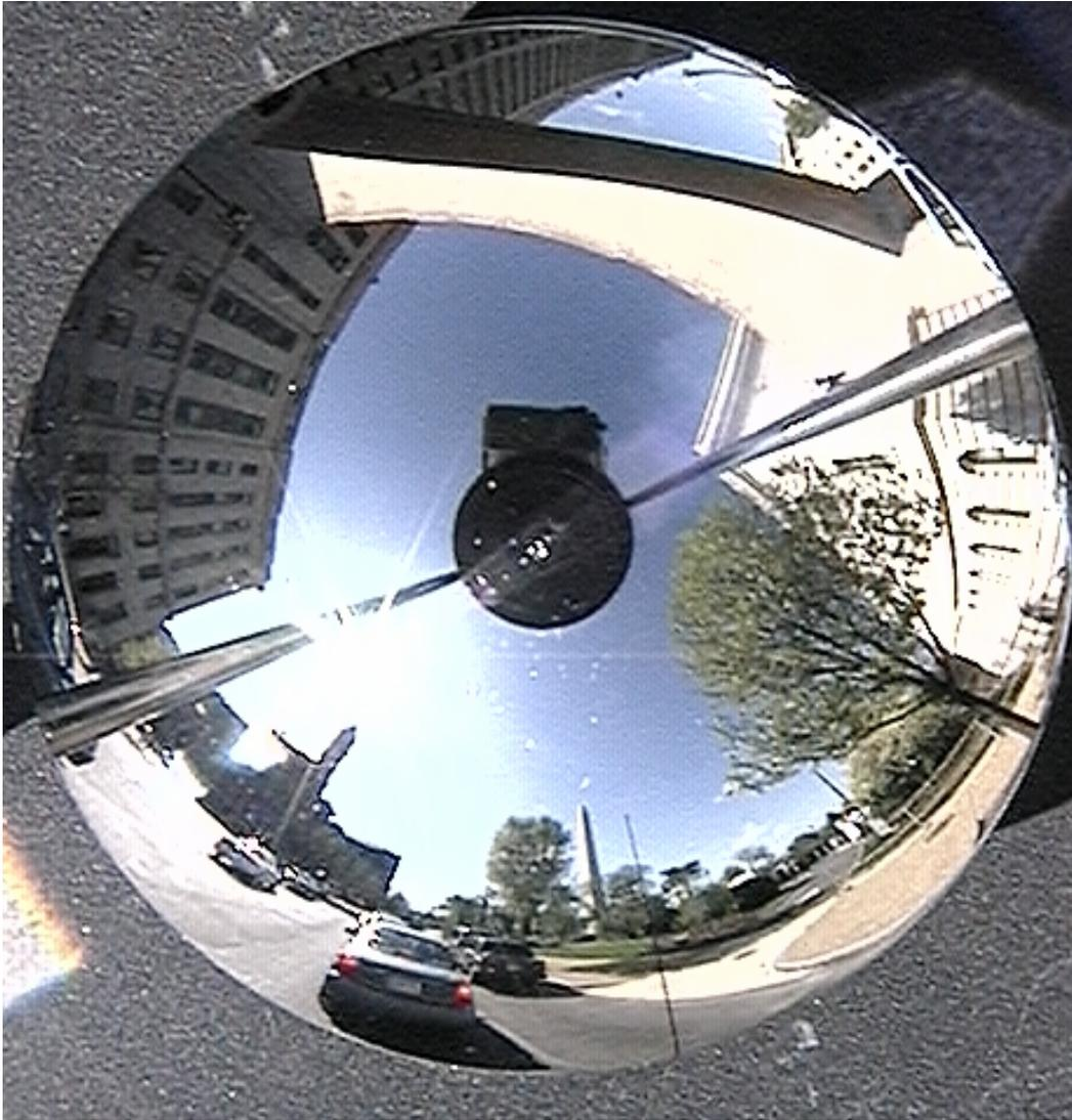
**Figure 3. An Omnidirectional (Paralmage) taken from a car. Note the “struts” are from an early version of the car mount, newer versions have only 1 (smaller) strut.**
