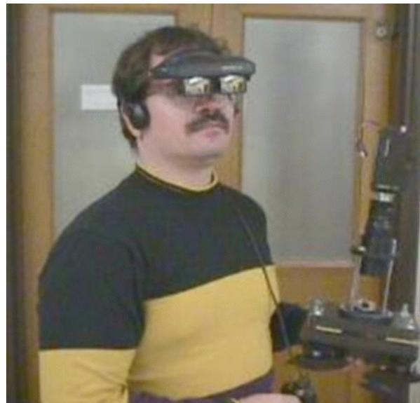
**Figure 4. An immersive interface: Remote Reality head-tracked HMD. User is holding an early car-mounted para-camera.**
