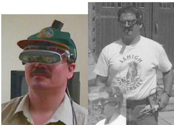
Fig. 5. Left is an immersive interface: Remote Reality head-tracked HMD and right is an informative monocular display with (a track-ball pointer).
