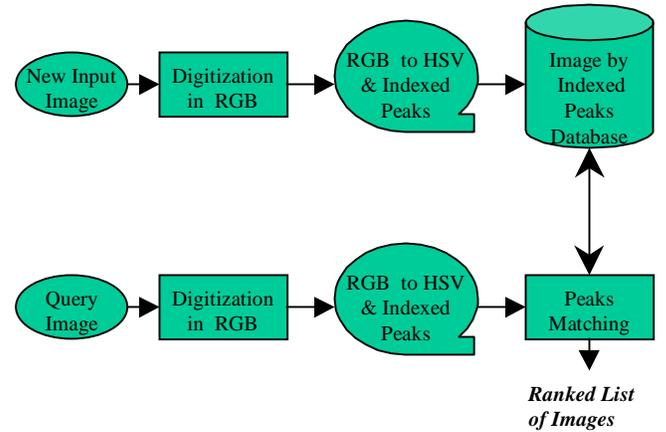
Fig. 1. A schematic histogram peak indexing system overview
