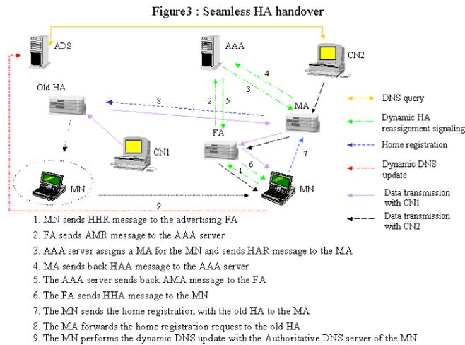
As illustrated in Figure 3, the MN is able to continue the communication with CN1 at the old home address and to start a new communication session with the CN2 directly at the new home address simultaneously after the seamless HA handover.
