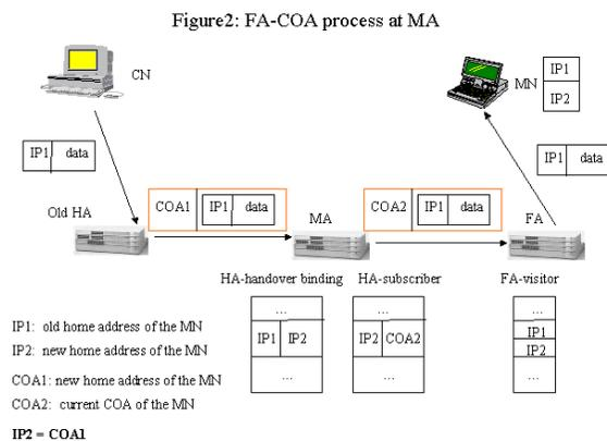
The MA could receive two kinds of the datagrams both destined to the new home address of the MN, one is encapsulated and
