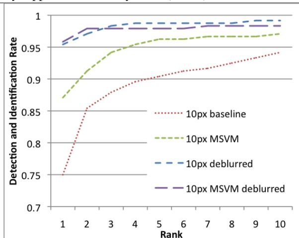
Fig. 5. Cumulative Match Curve for the 10-pixel blur case. This demonstrates how the method described in this paper forces the vast majority of its matches closer to Rank 1, whereas use of a single SVM creates a smoother curve, losing accuracy fairly consistently esp. in ranks 4 through 10. Note that the y-axis ranges from .7 to 1.0.
