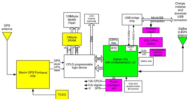
Figure 4 GeoZigBee Device Components
