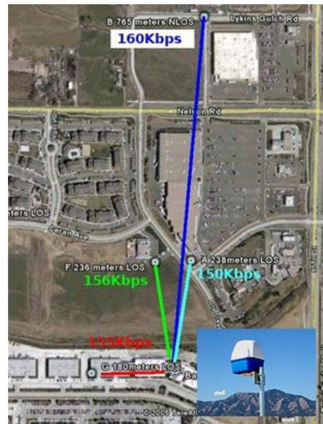
**Figure 3 Extended Range ZigBee Connection**
